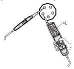
"L" signifies that the supposed phase L1 is the actual phase L2 and the supposed phase L2 is the actual phase L1.
