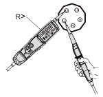
When re-testing with exchanged test probes the opposite symbol has to be illuminated.
