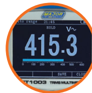
6000 Count 320 x 240 TFT colour LCD display
